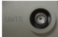
Fig 2.14 - GPRS antenna port
