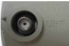
Fig. 2.13 - UHF antenna port
